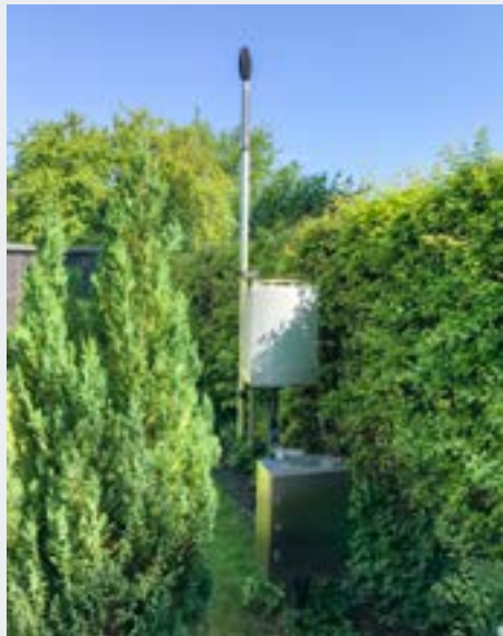
One of CPH's six noise-measuring stations located in residential areas around the airport.
