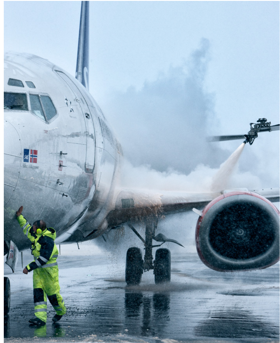
De-icing of aircraft removes snow and ice from the aircraft's wings to prevent ice formation on wings and flaps during take-off. De-icing is done just before take-off on platforms with collecting systems for the excess de-icing fluid.
